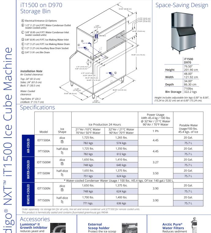
Order separately: Ice storage bin for all units, line-set and remote condenser unit JCT1500 for remote cooled units. This product is hermetically sealed and contains fluorinated greenhouse gas R404A
